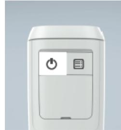
To turn the TRV on, short press the on/off button
