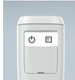
When in RF Comms Check, hold both buttons for 5 seconds
