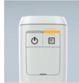
Right LED will flash amber for up to 2 minutes whilst binding
