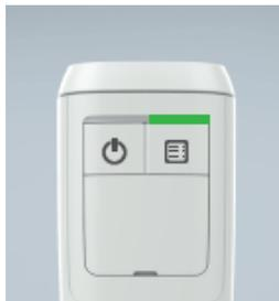
Successful binding is confirmed by right LED showing permanently green for 5 seconds
