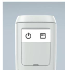
Press both buttons to check if TRV is locked
