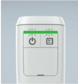
Once batteries are inserted the TRV confirms this by flashing both LEDs green for 5 secs
